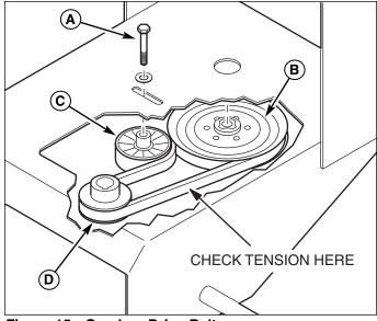
Figure 15. Gearbox Drive Belt
